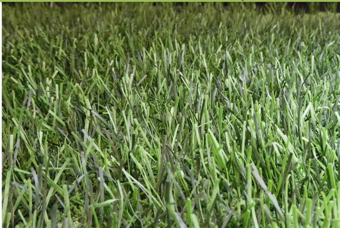
Fig. 18: DOMO Duraforce XSL after 160,000 cycles at the Lisport wear tester
