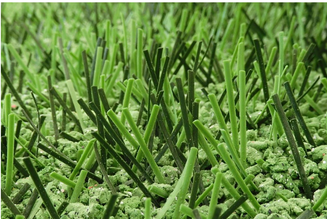
Fig. 7: DOMO Duraforce XSL after 40,000 cycles at the Lisport wear tester
