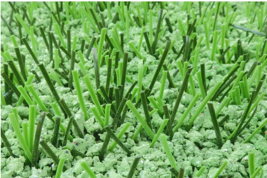
Fig. 3 DOMO Duraforce XSL at the start of the test
