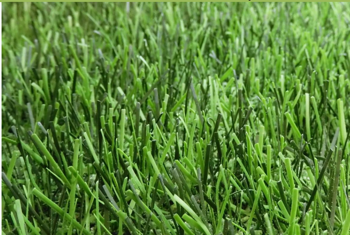
Fig. 14: DOMO Duraforce XSL after 120,000 cycles at the Lisport wear tester
