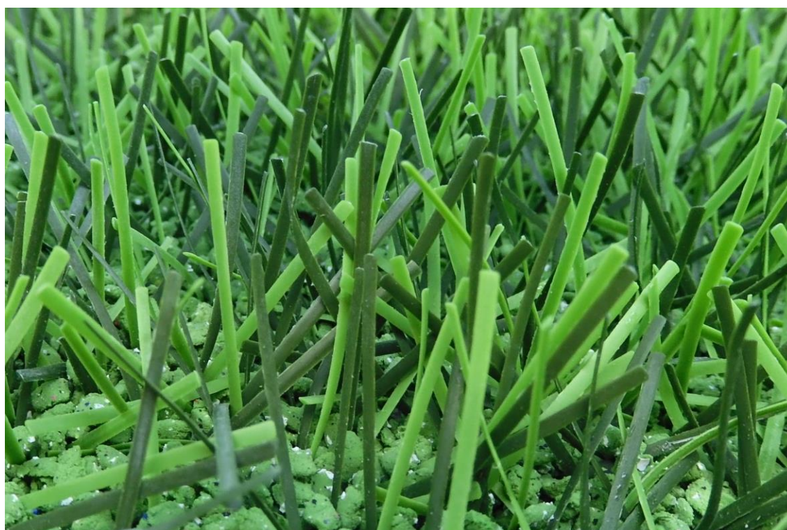
Fig. 13: DOMO Duraforce XSL after 100,000 cycles at the Lisport wear tester
