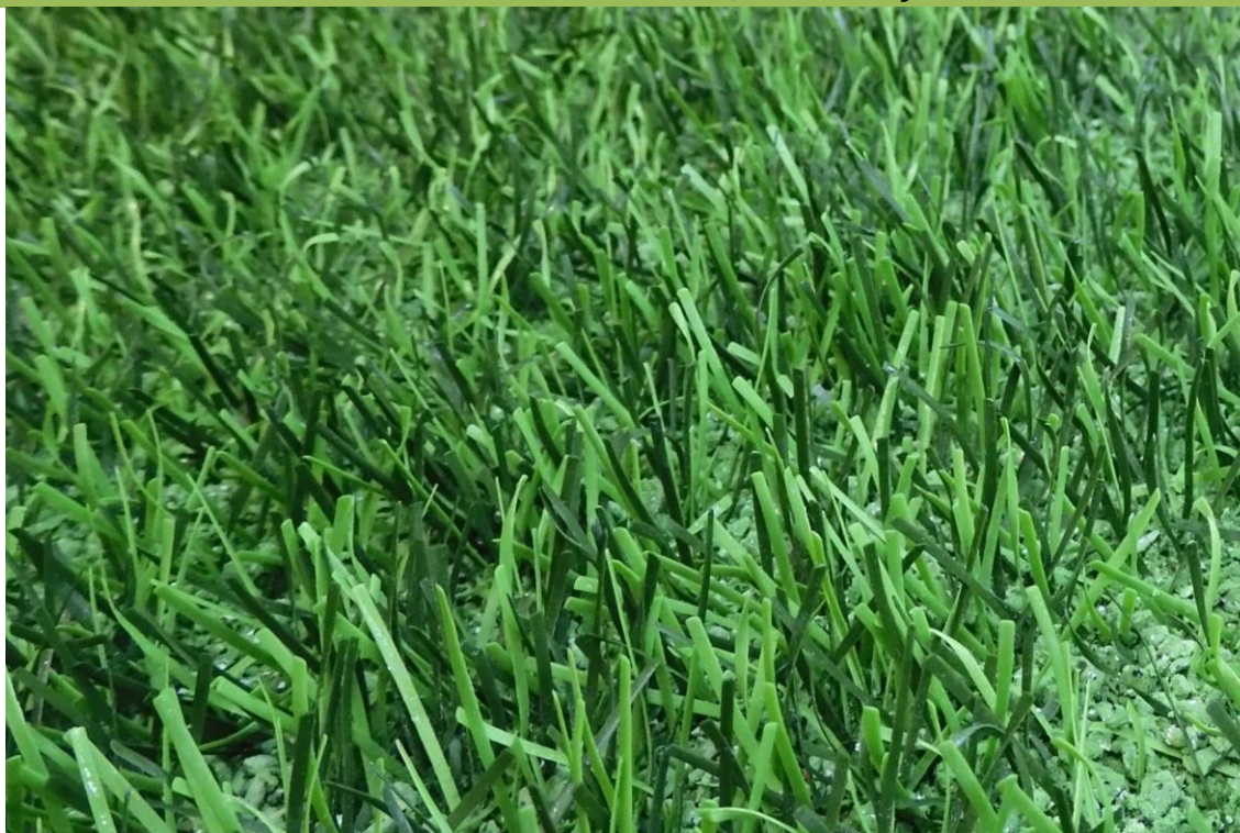
Fig. 20: DOMO Duraforce XSL after 180,000 cycles at the Lisport wear tester
