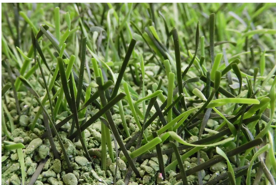
Fig. 31: DOMO Duraforce XSL after 280,000 cycles at the Lisport wear tester
