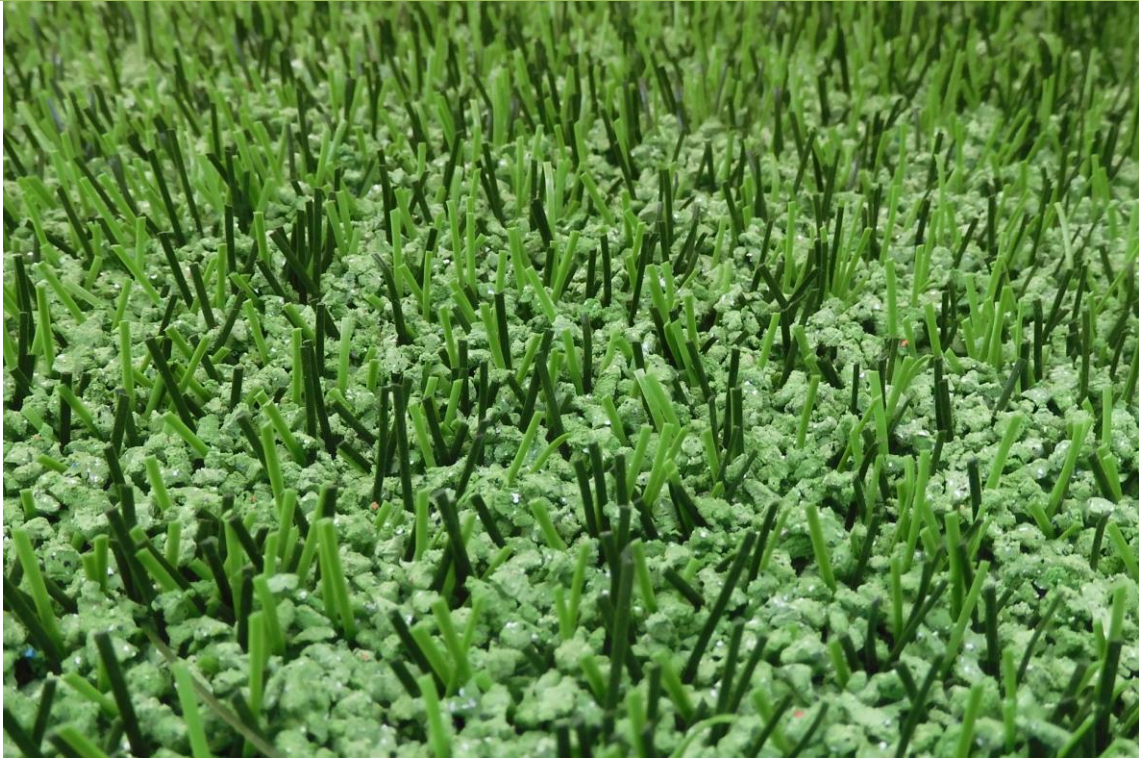
Fig. 2: DOMO Duraforce XSL at the start of the test
