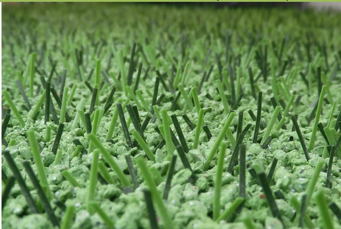
Fig. 4: DOMO Duraforce XSL after 20,000 cycles at the Lisport wear tester
