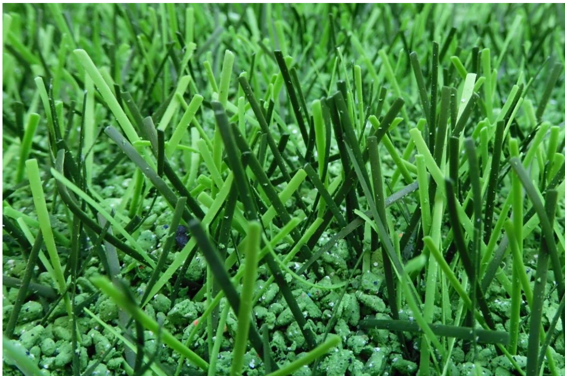
Fig. 17: DOMO Duraforce XSL after 140,000 cycles at the Lisport wear tester
