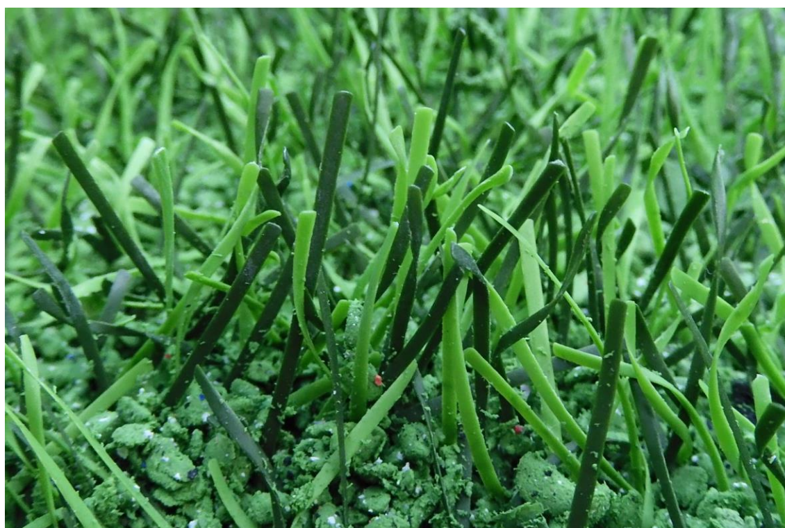
Fig. 25: DOMO Duraforce XSL after 220,000 cycles at the Lisport wear tester
