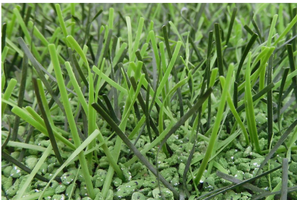
Fig. 27: DOMO Duraforce XSL after 240,000 cycles at the Lisport wear tester
