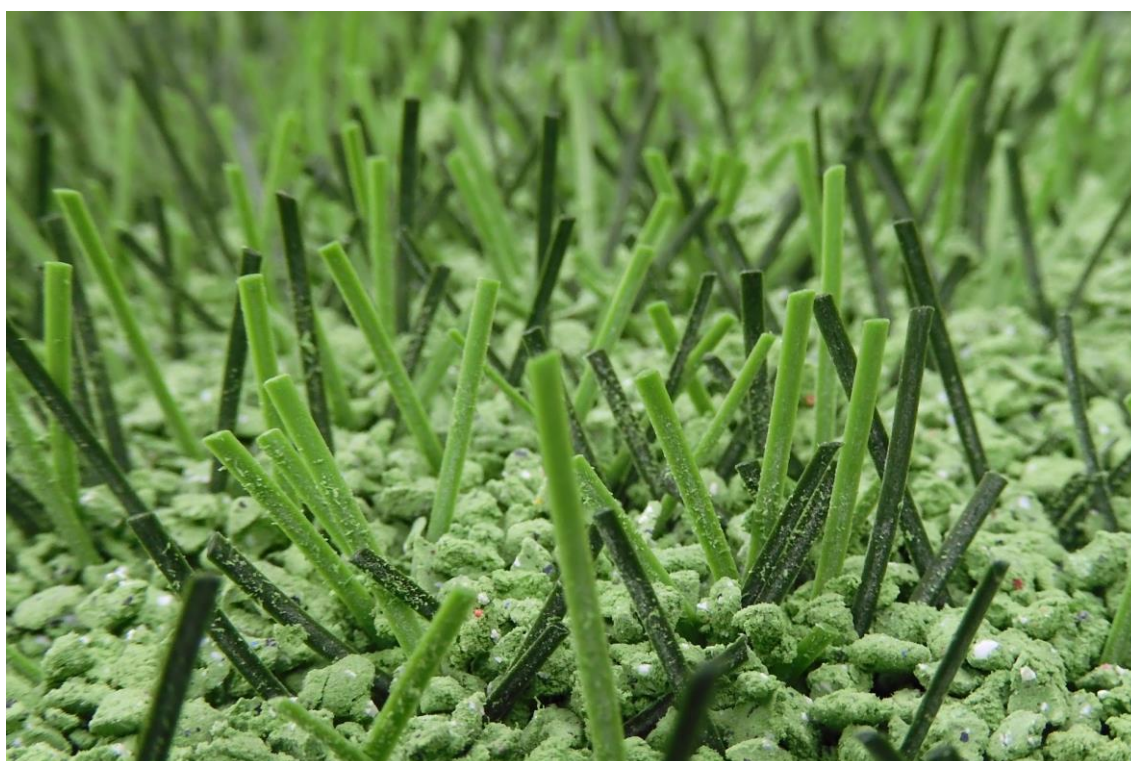
Fig. 5: DOMO Duraforce XSL after 20,000 cycles at the Lisport wear tester
