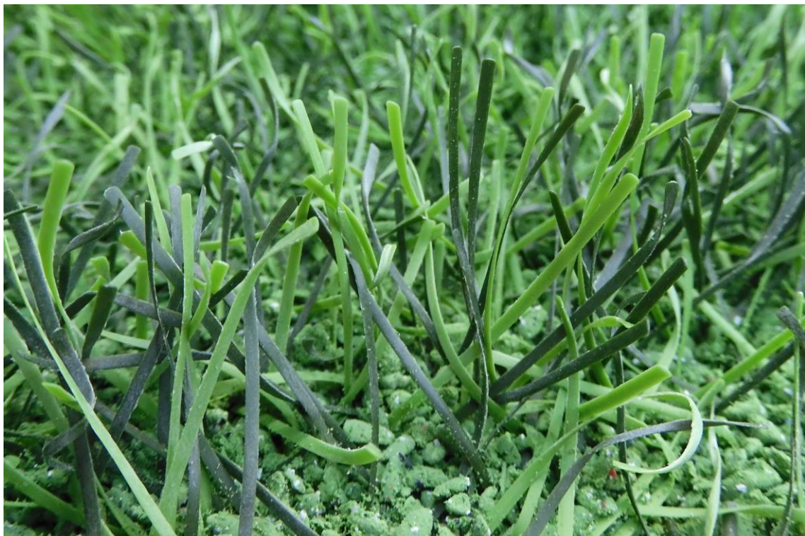
Fig. 33: DOMO Duraforce XSL after 300,000 cycles at the Lisport wear tester
