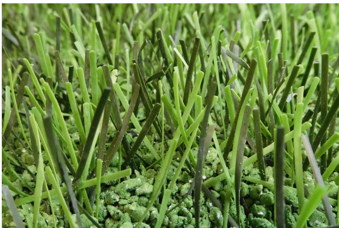
Fig. 19: DOMO Duraforce XSL after 160,000 cycles at the Lisport wear tester
