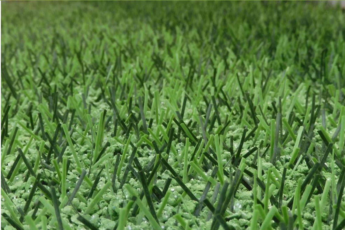
Fig. 6: DOMO Duraforce XSL after 40,000 cycles at the Lisport wear tester
