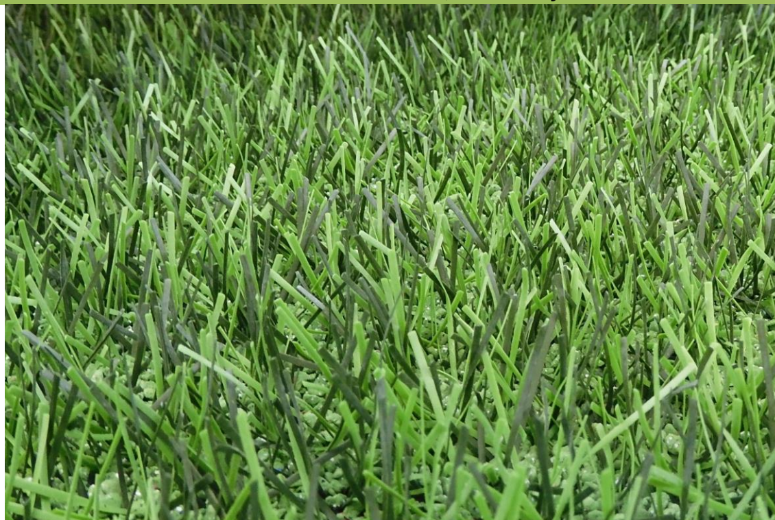
Fig. 12: DOMO Duraforce XSL after 100,000 cycles at the Lisport wear tester
