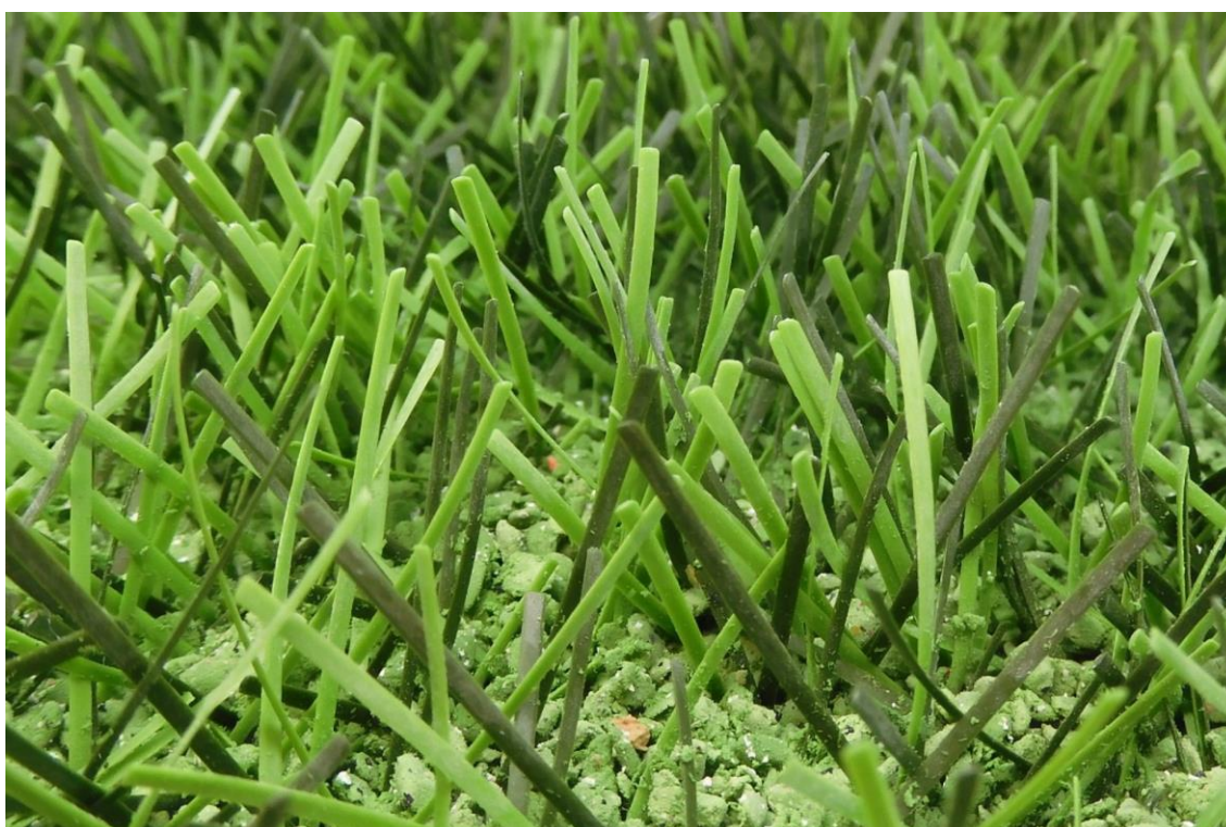
Fig. 15: DOMO Duraforce XSL after 120,000 cycles at the Lisport wear tester
