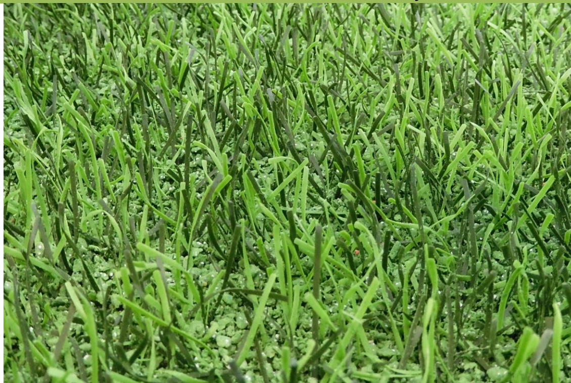
Fig. 22: DOMO Duraforce XSL after 200,000 cycles at the Lisport wear tester
