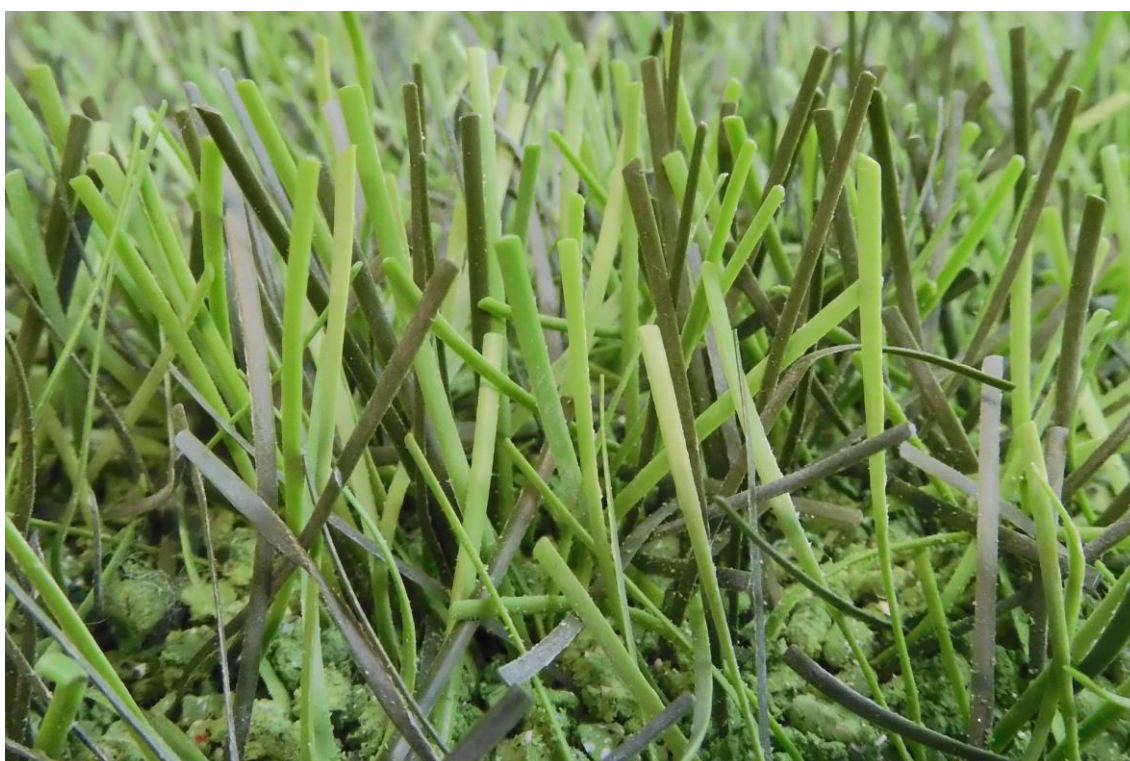
Fig. 11: DOMO Duraforce XSL after 80,000 cycles at the Lisport wear tester
