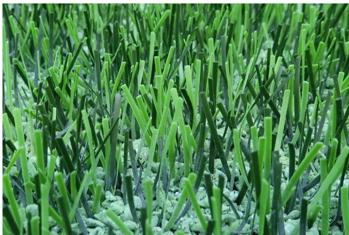
Fig. 9: DOMO Duraforce XSL after 60,000 cycles at the Lisport wear tester
