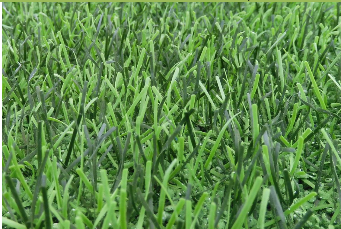
Fig. 26: DOMO Duraforce XSL after 240,000 cycles at the Lisport wear tester
