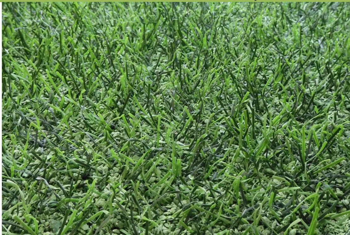
Fig. 30: DOMO Duraforce XSL after 280,000 cycles at the Lisport wear tester
