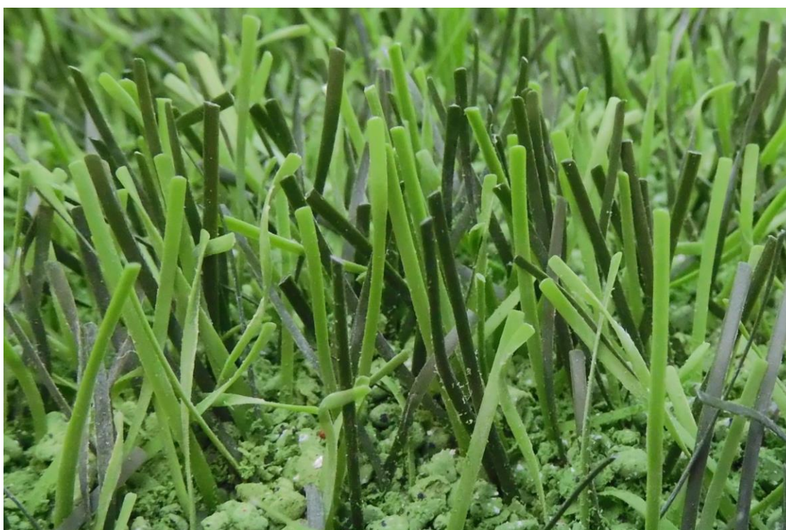
Fig. 21: DOMO Duraforce XSL after 180,000 cycles at the Lisport wear tester
