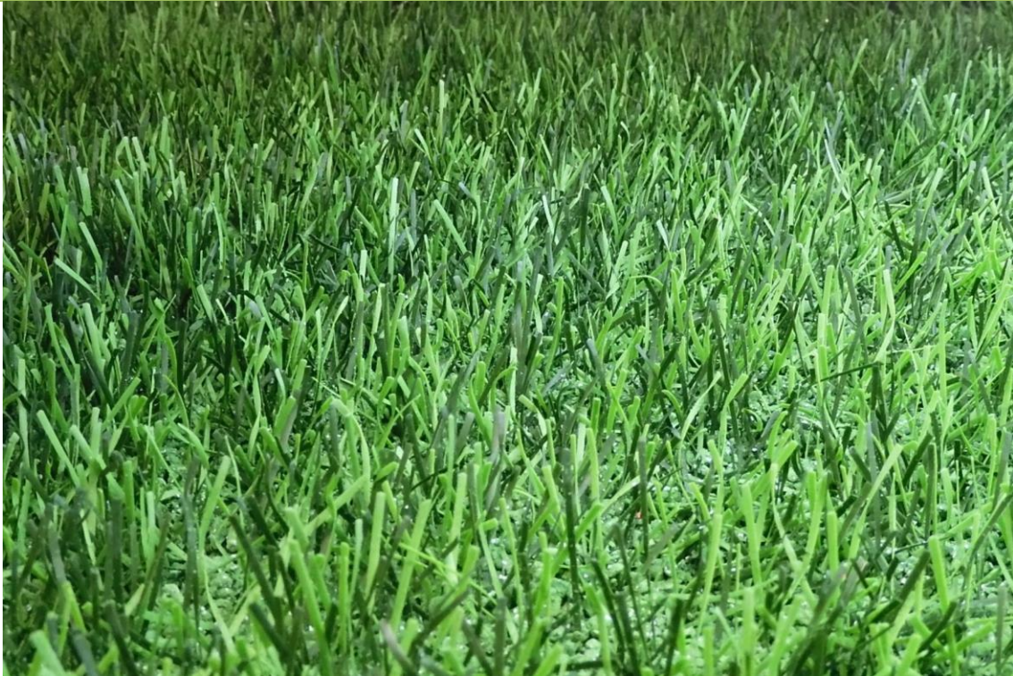
Fig. 16: DOMO Duraforce XSL after 140,000 cycles at the Lisport wear tester
