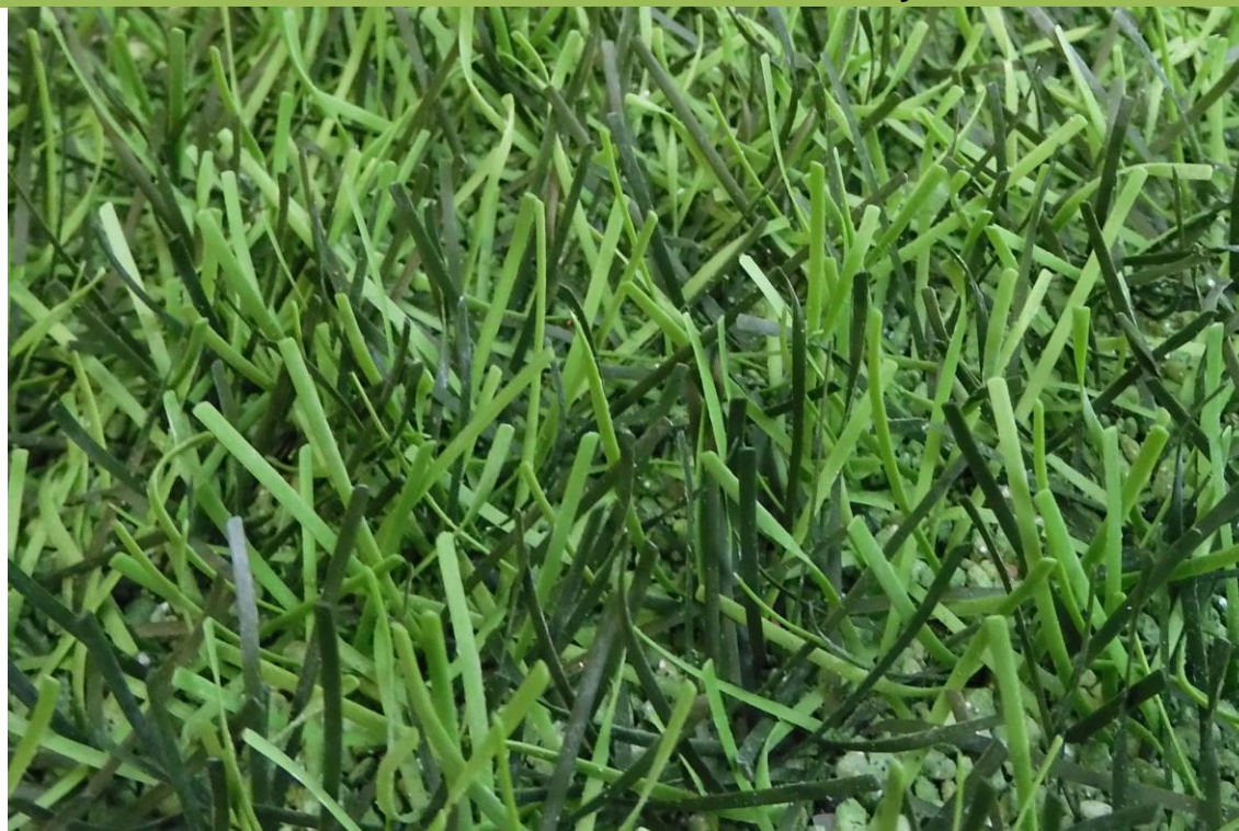
Fig. 24: DOMO Duraforce XSL after 220,000 cycles at the Lisport wear tester
