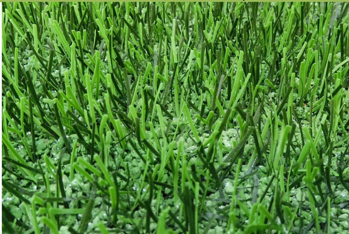
Fig. 8: DOMO Duraforce XSL after 60,000 cycles at the Lisport wear tester
