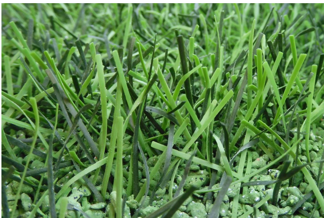
Fig. 23: DOMO Duraforce XSL after 200,000 cycles at the Lisport wear tester
