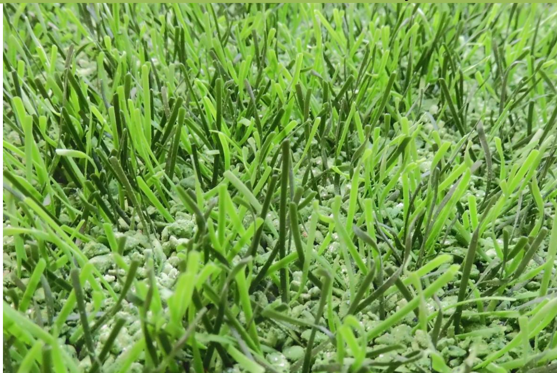
Fig. 28: DOMO Duraforce XSL after 260,000 cycles at the Lisport wear tester
