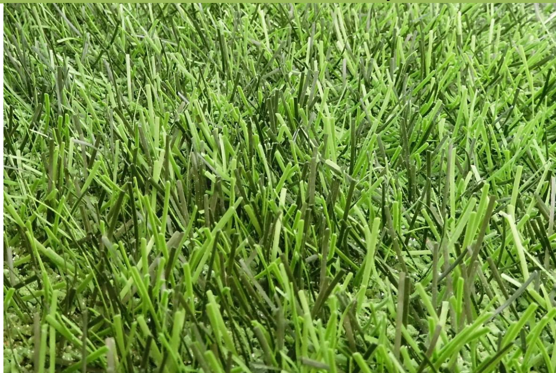
Fig. 10: DOMO Duraforce XSL after 80,000 cycles at the Lisport wear tester
