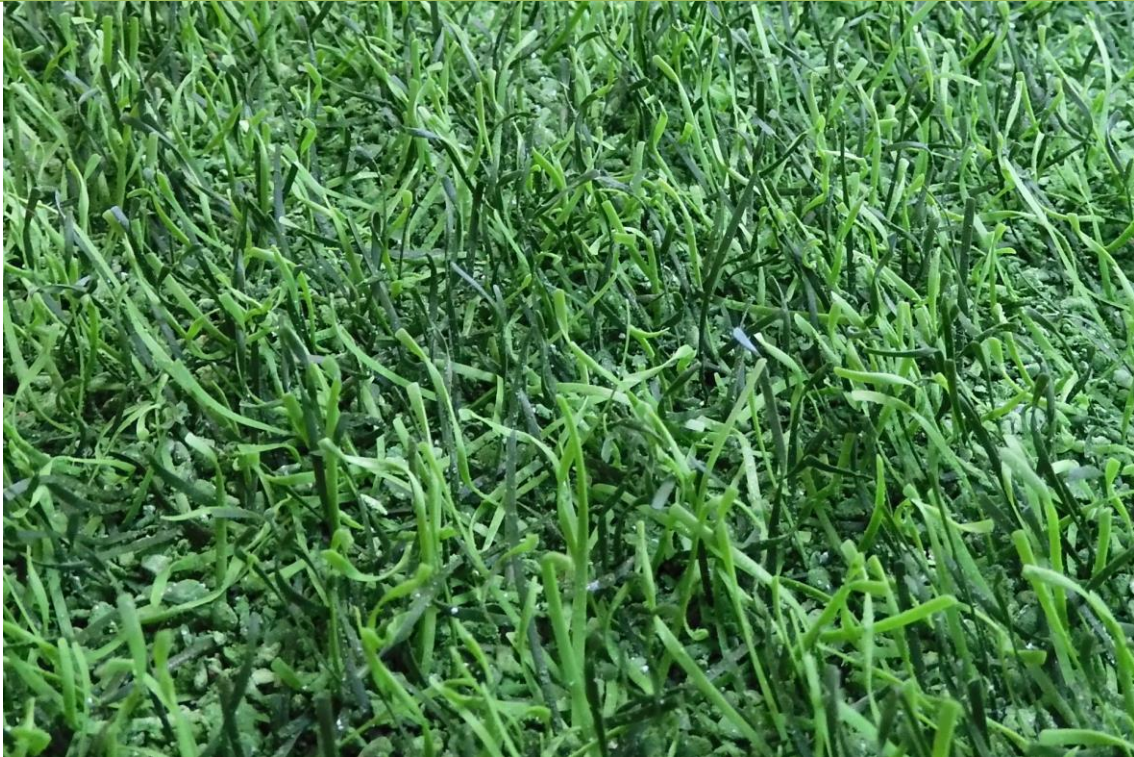
Fig. 32: DOMO Duraforce XSL after 300,000 cycles at the Lisport wear tester
