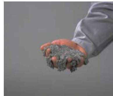
The compound is too wet. Discard the compound
